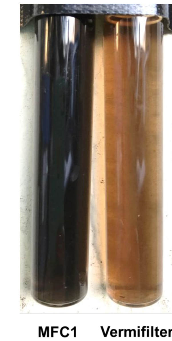
Fig. 3. Concentrations of soluble organics (sCOD) in water flowing through the Vintners Square treatment system. Left: Progressive decreasing trend of sCOD traces found in WW Right: Relative clarity of MFC1 effluent compared to effluent from the vermifilter.
