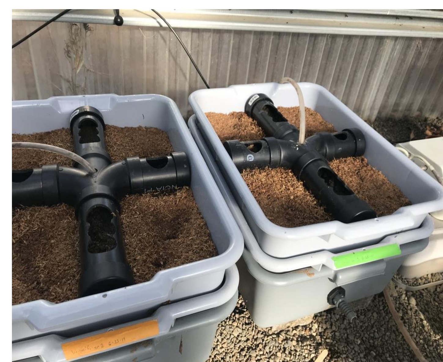
Fig. 4. Left: Filters containing a peat:cedar-rice bran bed medium with sand distributor of winery wastewater. Stackable cedar-rice bran "enzyme bath" bed medium placed on top previous vermifilter to promote worm migration Right: Photo inset: Red earthworm ( Eisenia fetida ).
